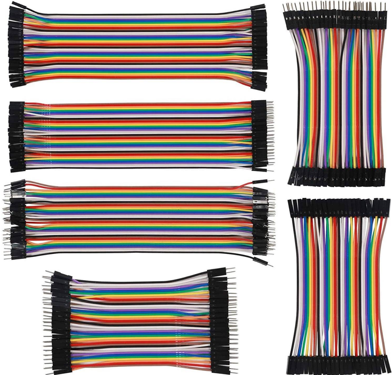
Types of Jumper wires which consist of Male to Male, Female to Female, Male to Female connectors.
